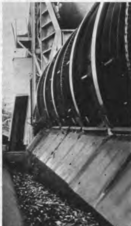
Fig. 5. All of the bark, here being removed in Jari's debarker, is still burned. Since nutrients are concentrated in the bark, most are lost from the system.
