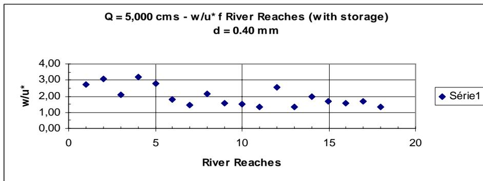
0.30 mm particles are moving in saltation up to RR 5 further upstream they are moving in suspension over the remaining length of the pool.
