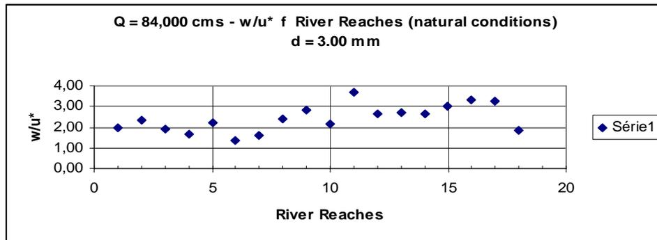
**2.2 Sediment transport characteristics with Storage (Ponding) at AHE Santo Antônio for the following river discharges: 5,000; 10,000; 18,000; 39,100; 48,600; 61,200; 2,600 and 84,000 m<sup>3</sup>/s**
