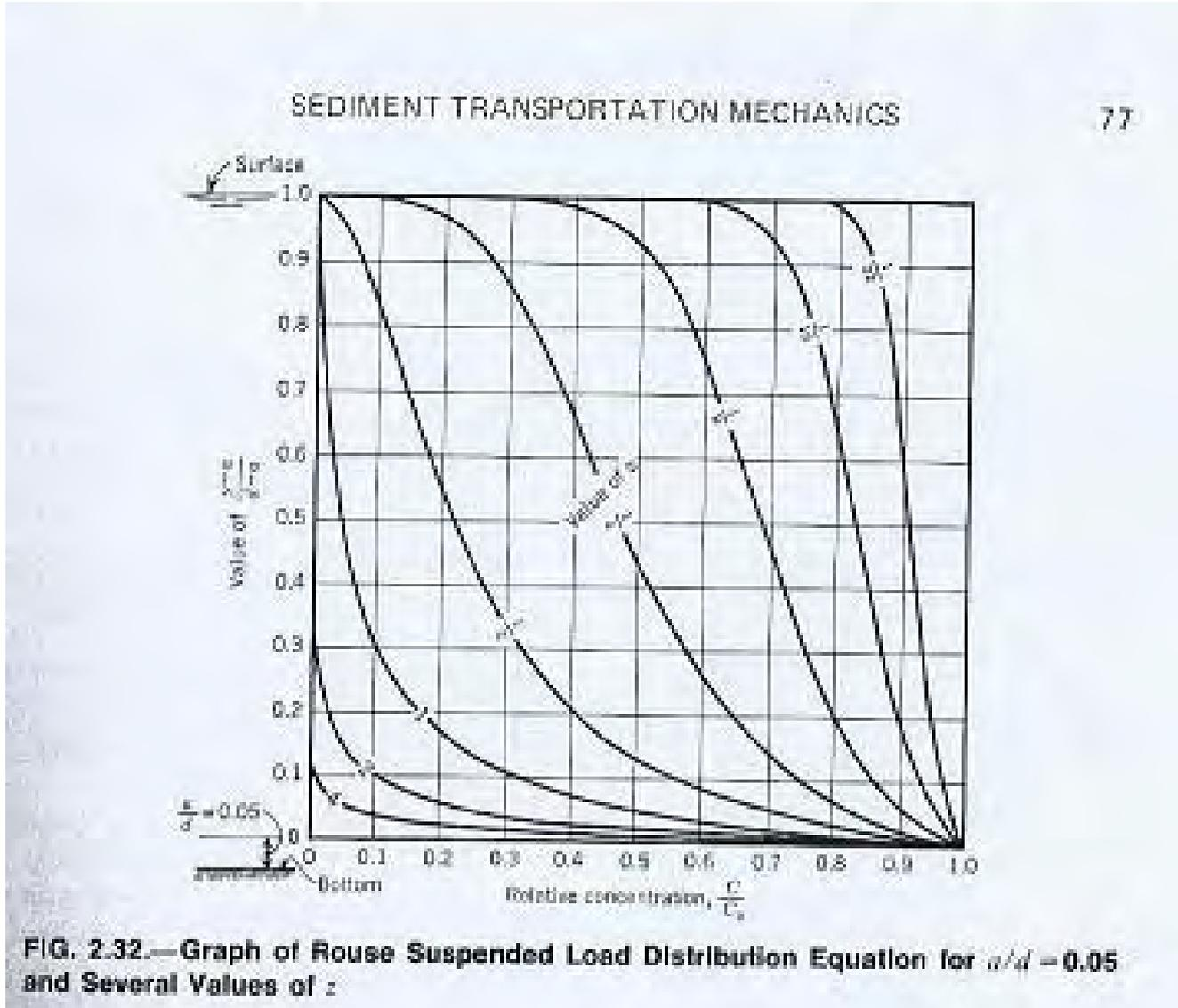
**Figure 2.1 –Graph of Rouse Suspended Load Distribution Equation for  $a/d$  0.05
